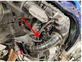
Locate 2pin sealed connector of the 12V car plug power connector and plug Dongle in between.
