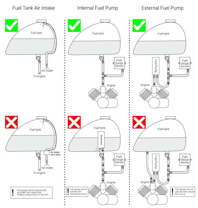
**CAUTION**: We cannot guarantee the correct function on all motorcycles with a fuel pump. The external fuel pump may cause problems with measuring on some motorcycles. If this problem occurs, you can return FuelGauge to us and we will return your money back to you. Device must be in intact condition.
