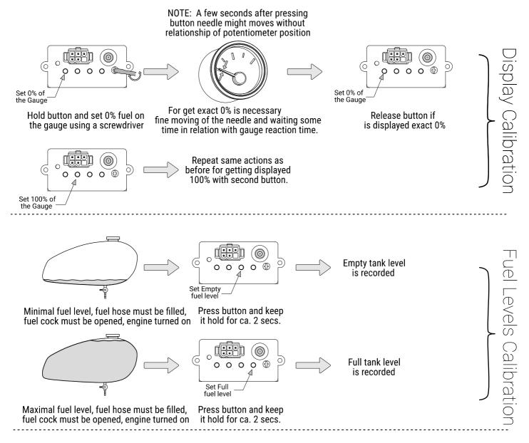
Display Calibration is independent to Fuel level calibration, each of them are able to calibrate separately.
